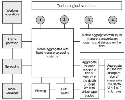
Fig. 1. Technological versions of liquid manure transportation and incorporation chosen for comparison
